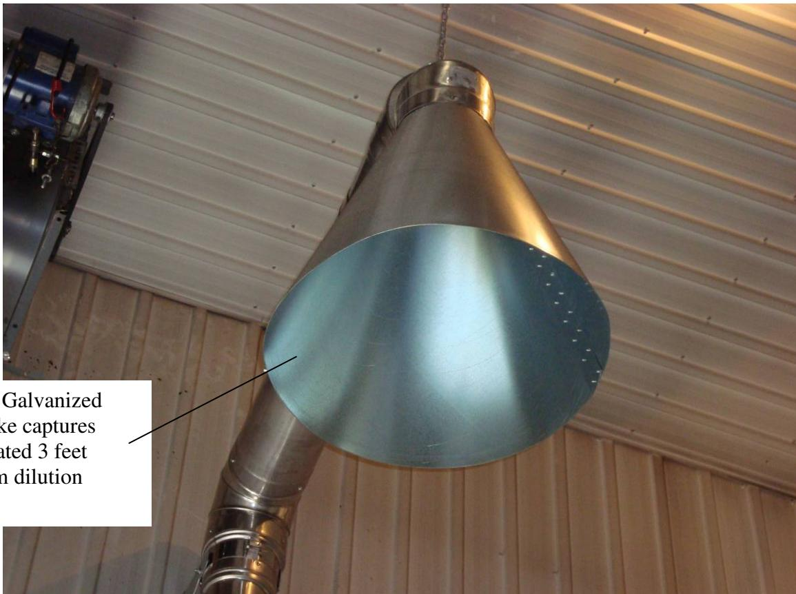
24in. dia. Galvanized steel smoke captures hood, located 3 feet away from dilution tunnel
