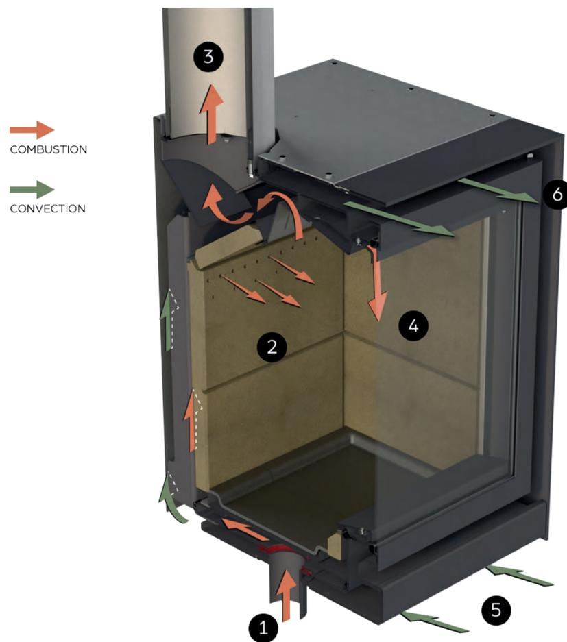
**1** The air required for combustion comes directly from under through an outside air intake connector specially designed for the Stûv 16-in, Z and combo models.
